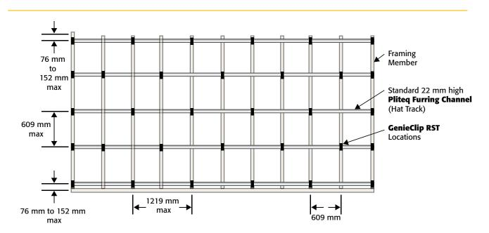
Wall or Ceiling Framing at 406 mm o.c.
